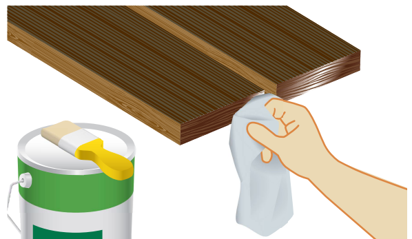
2.3. Applying oil to the burned surface
